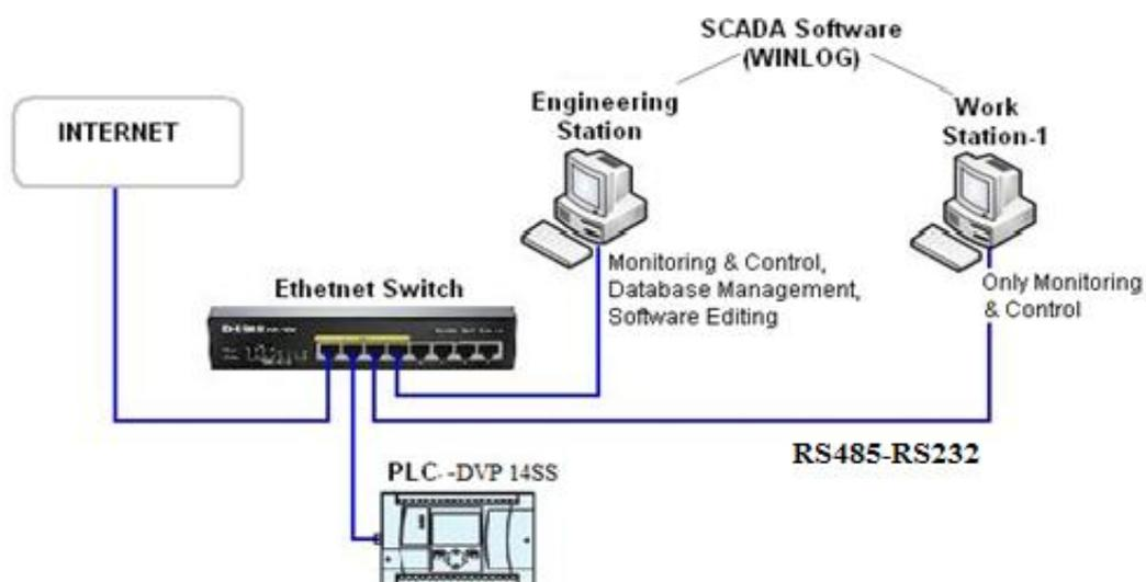
Fig 2. Interfacing of PLC with SCADA
