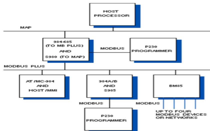
Fig.3. Overview of Modbus Protocol Application [7]
