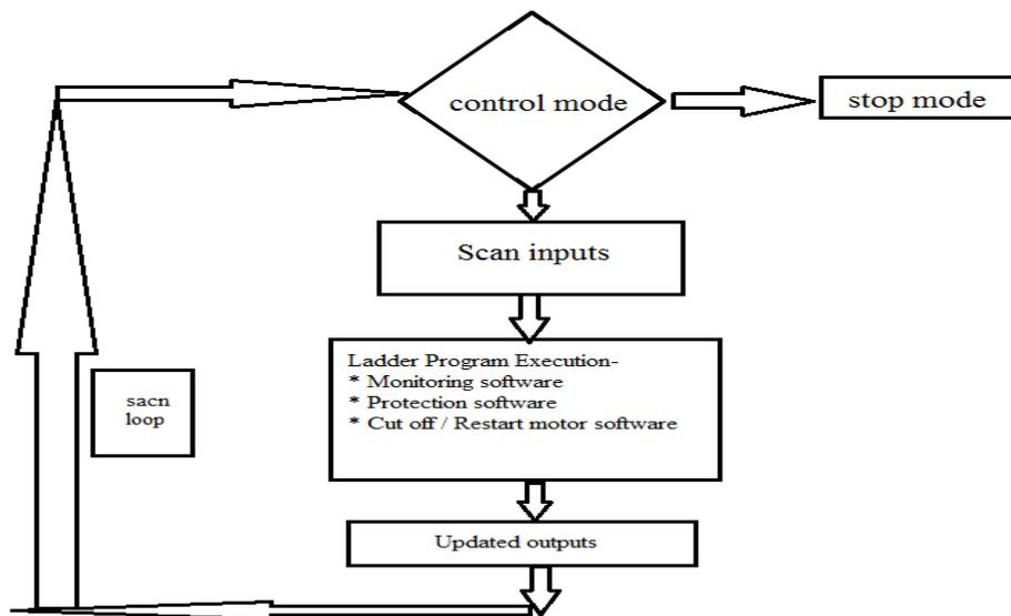
Fig.4 flowchart of the Main Block Diagram
