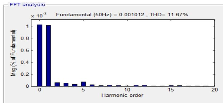
Fig.11 FFT analysis of ZSI fed IM drive
