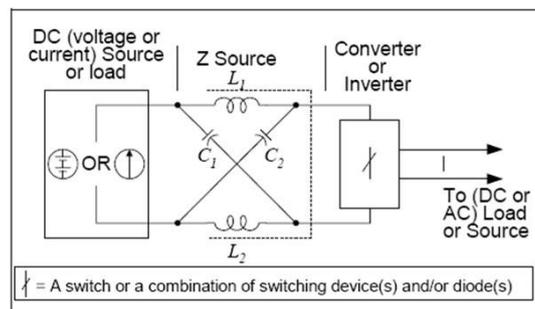
Fig. 2 Z-Source Inverter
