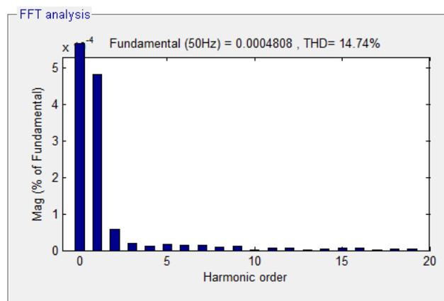
Fig.9 FFT analysis of CSI fed IM drive
