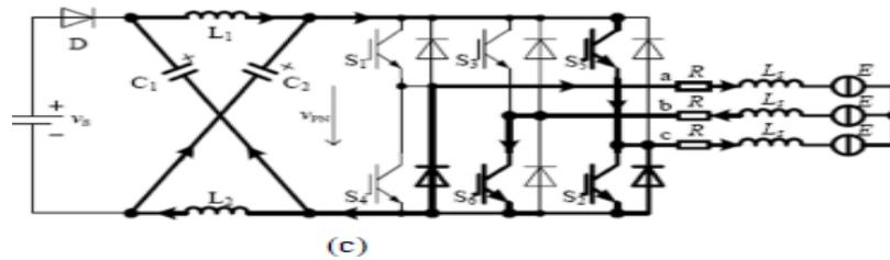
Fig. 4 Equivalent circuit during Phase commutation stage: (a) Open (b) Active (c) Shoot-through state
