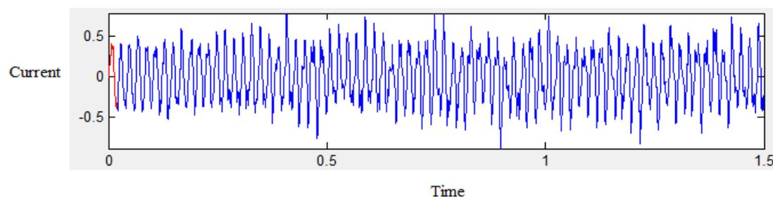
Fig.8 Inverter output 3-phase current waveform
