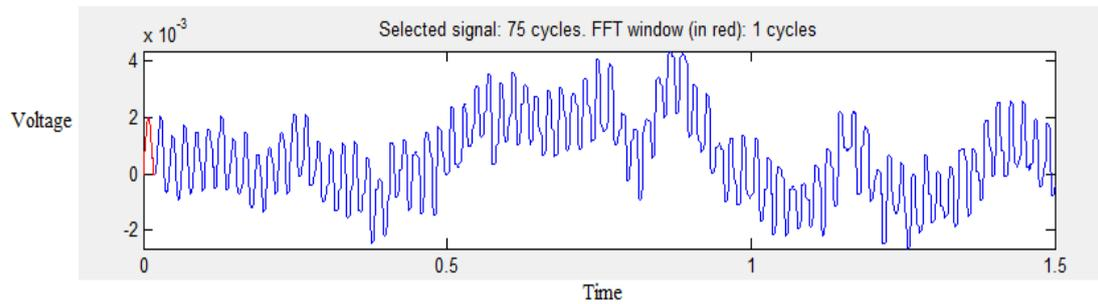
Fig.7 Inverter output 3-phase output voltage waveform
