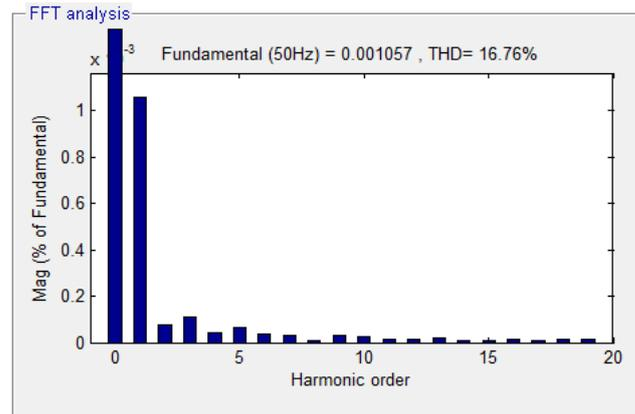
Fig.10 FFT analysis of VSI fed IM drive
