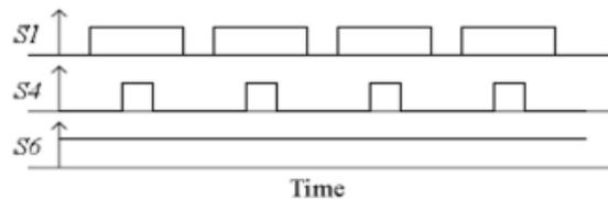
Fig. 5 Waveform of the Gate signal
