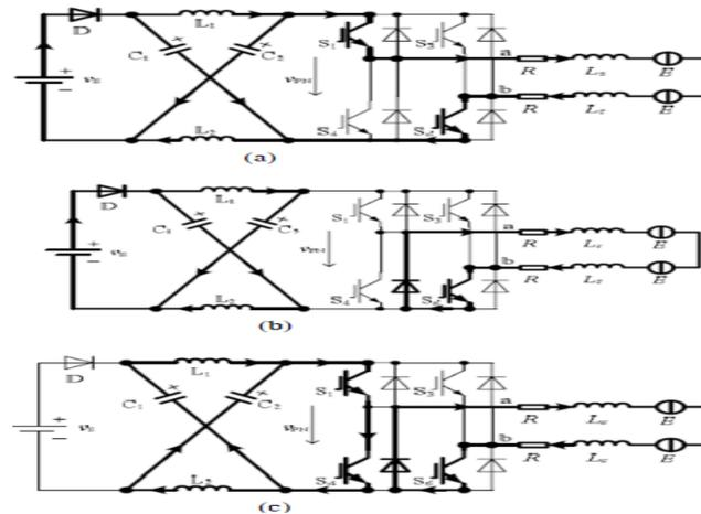
Fig 3. Equivalent circuit during non-commutation stage: (a) Open (b) Active (c) Shoot – through.
