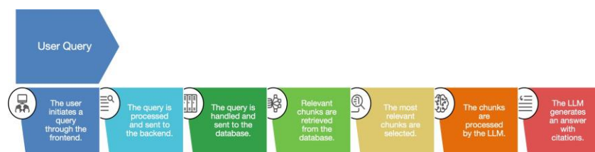
Fig. 1. System Architecture of RAG-Based Geoscience Assistant
