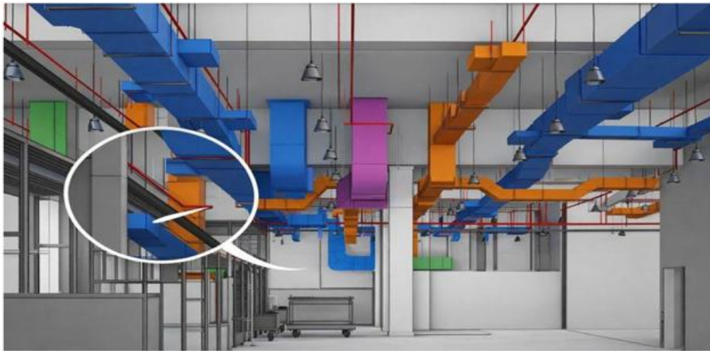
Fig. 1: Building system clash detection visualization
