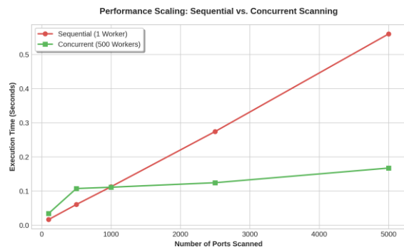
Fig. 3. Performance Scaling: Execution times of single-threaded vs. con-current (500 workers) scanning.
