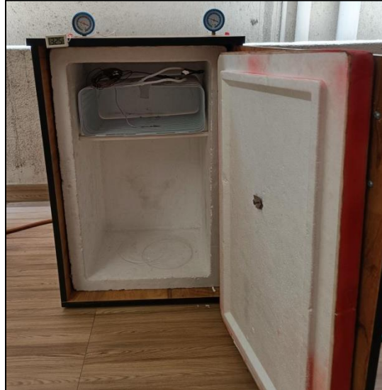
Fig.9: Construction of the LPG refrigerator
