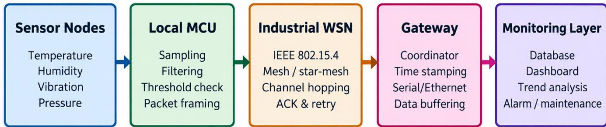
Figure 1. Proposed WSN architecture for industrial monitoring applications.
