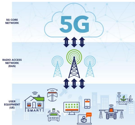
Fig.1: End-to-End Overview of the 5G Network Architecture
