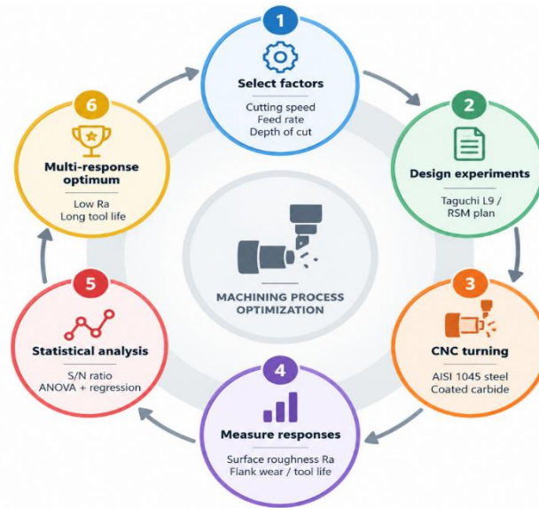
Figure 1. Step-by-step workflow for CNC turning parameter optimization.
