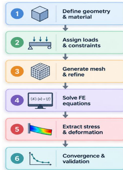
Figure 1. Step-by-step finite element methodology used for stress and deformation assessment.
