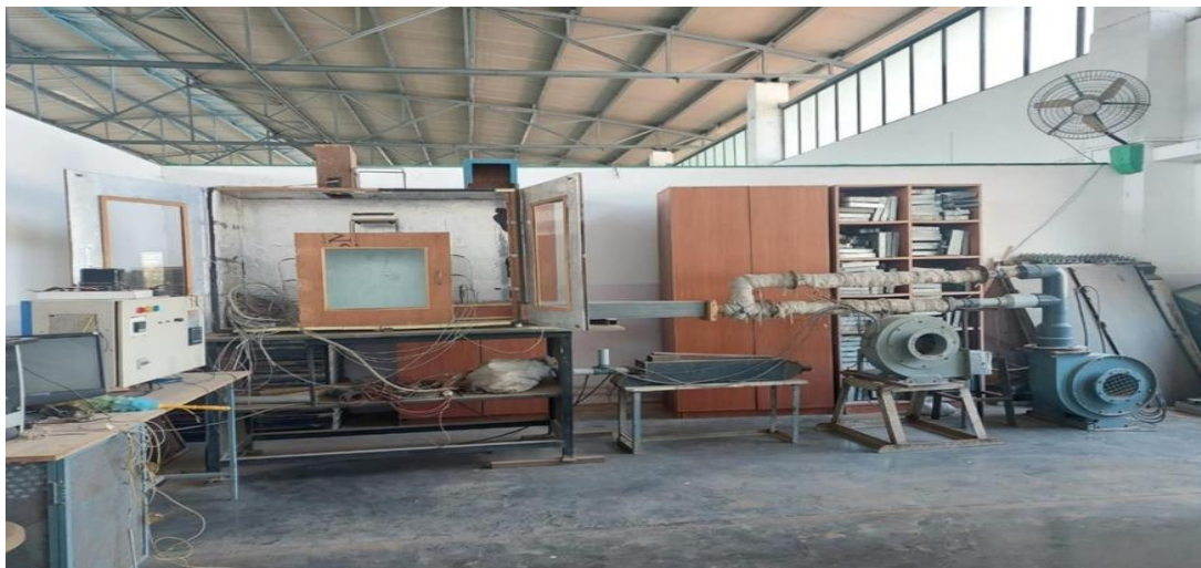
Fig. 9. Fully operational physical experimental setup showing the centrifugal blower, heating ductwork, insulated wooden drying chamber, instrumentation, and control unit.
