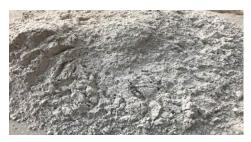
**Virgin Fly Ash** is collected from Koradi Power Plant. It is a fine powder produced from burning coal in thermal power stations. It mainly contains silica, alumina, and iron oxides, which help improve soil properties.
