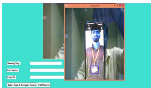
Figure 2: No ID Card Detected Displays warning message, predicted roll number, and email entry field.
