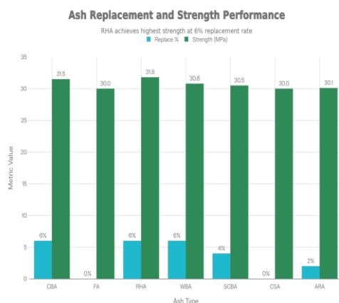
Graph 2: Optimal Replacement Percentages and Peak Compressive Strengths for M30 Grade Concrete
