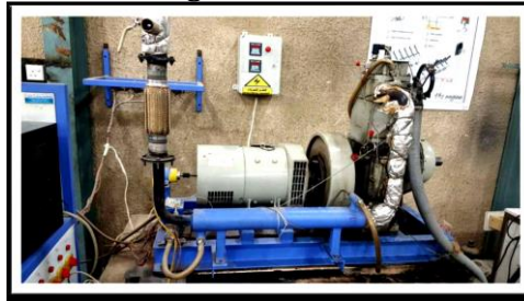
Figure 3: The diesel engine experimental setup (front view)
