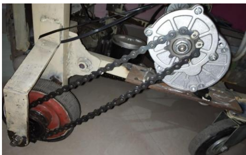
Fig. 1: Chain Drive with chain and sprocket
