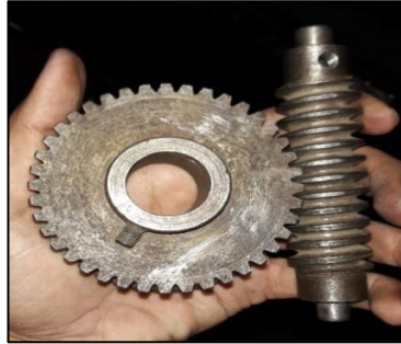
Fig 4: Worm and Worm Gear Arrangement
