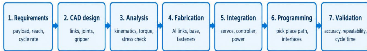
Figure 1. Step-by-step methodology for design, fabrication, control integration, and validation.
