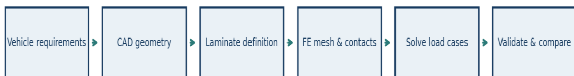
Figure 1. Step-by-step finite element methodology for the composite leaf spring.
