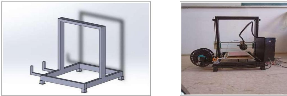
Fig. 3. Redesigned frame and completed IoT-enabled FDM printer.
