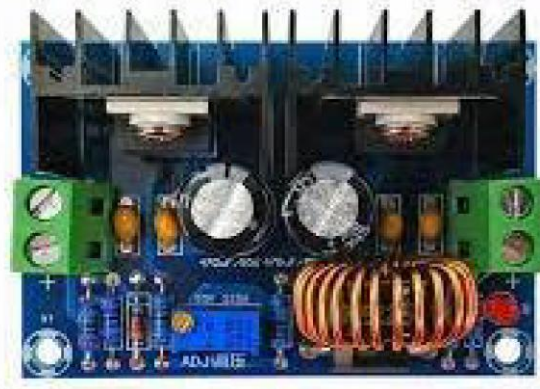
Fig. 9. XL4016 PWM step-down DC-DC buck converter module.
