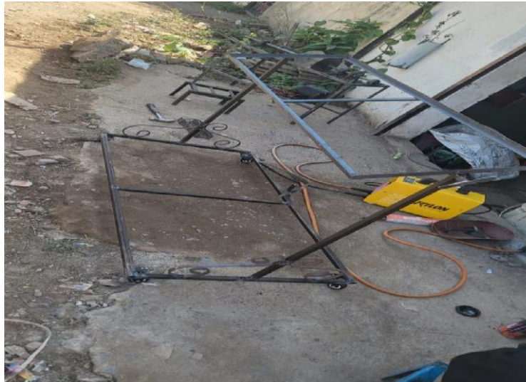
Fig. 2. Fabricated Plain Carbon Steel frame structure.
