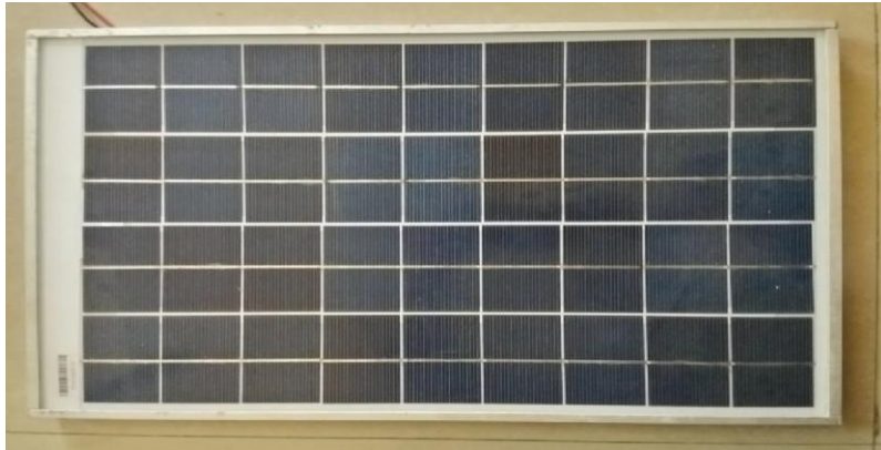
Fig. 6. Polycrystalline solar panel module.
