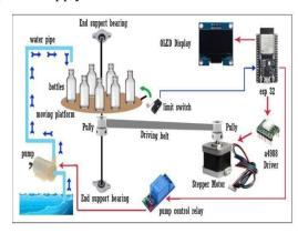
Circuit Design and Integration: The electrical circuit was designed to interface all components with the microcontroller. Sensor outputs are connected to the microcontroller inputpins, while output pinscontrolthesolenoid valve and conveyor motor through a relay or driver circuit.
