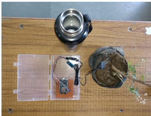
Figure 7 : Real – Time Soil Moisture Sensor Testing in Soil and Saltwater
