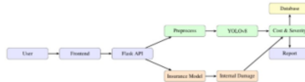
Fig. 1. Proposed system architecture showing interaction between the user frontend, Flask API, AI/ML components, database, and report generation module.
