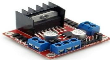
Fig 3. L298N Motor Driver
