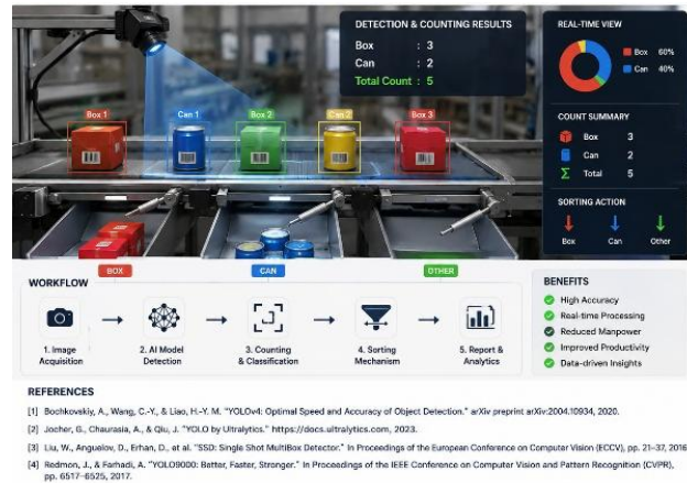
Fig 1. AI-Based Product Object Detection, Counting, and Sorting System Workflow and Real-Time Monitoring Dashboard
