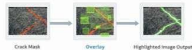
Fig. 4. Crack Visualization Using Mask Overlay Technique
