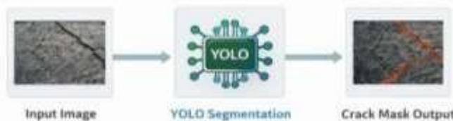
Fig. 3. YOLO-Based Crack Segmentation and Mask Generation
