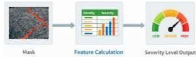
Fig. 5. Crack Feature Extraction and Severity Classification
