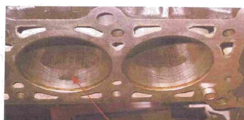
Scores, pits, and scratches
