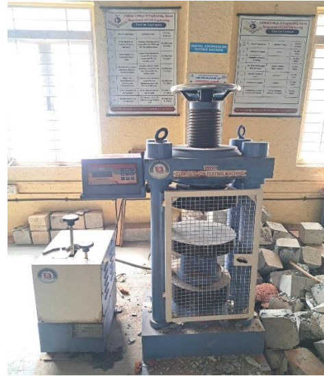
Fig 4 Compression testing machine
