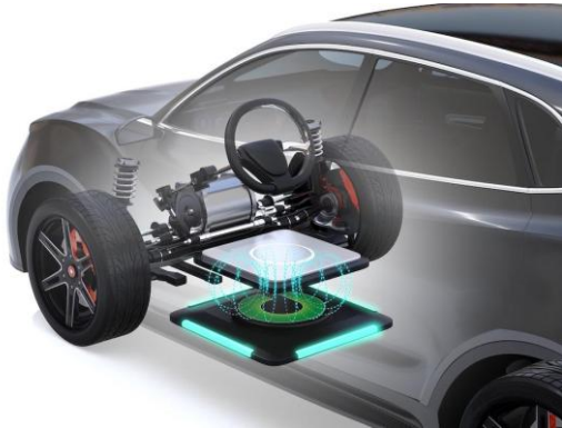
Figure 5: Field coupling between the ground-based transmitter coil and the vehicle-mounted receiver coil, shown in side cutaway.
