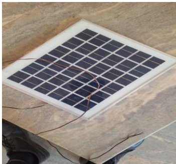
Figure 8: Solar panel providing supplementary supply to the charging arrangement.
