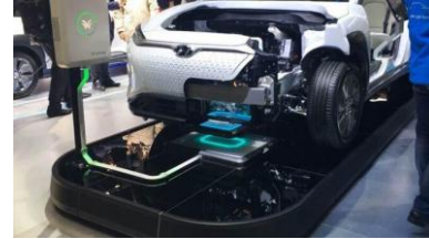
Figure 7: Wireless charging station arrangement.
