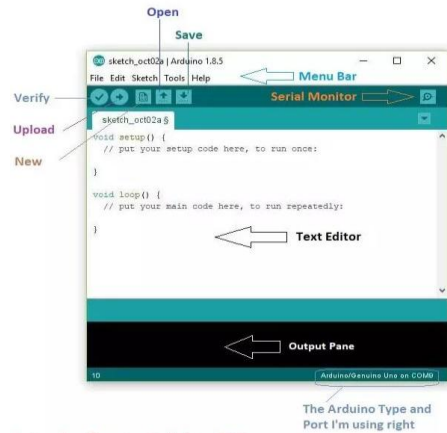
Figure 10: Arduino IDE development environment used for firmware compilation and upload.
