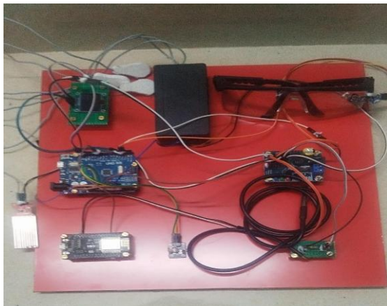
Figure 12: Experimental setup of the assembled prototype with all five sensing channels, the Arduino acquisition unit and the ESP8266 uplink.
