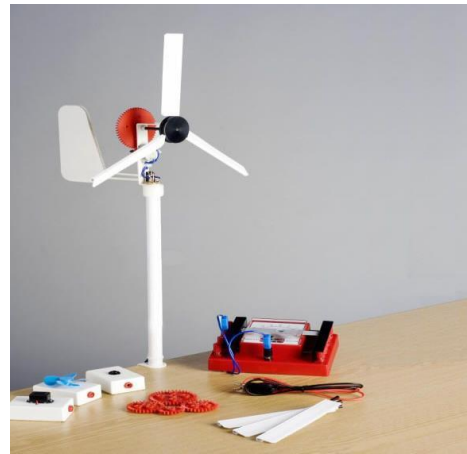
Figure 3: Laboratory kit comprising the small wind turbine and photovoltaic panel used in the experimental arrangement.
