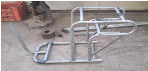
Figure 19: Welded frame during fabrication.
