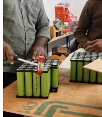
Figure 21: Battery pack assembly from individual cells.
