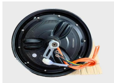
Figure 6: Hub motor integrated into the wheel.
