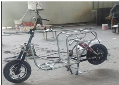
Figure 20: Rolling chassis with wheels and running gear mounted.
