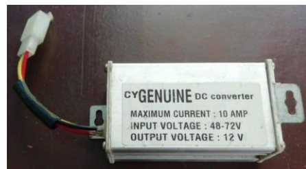
Figure 11: DC–DC converter stepping traction voltage down to 12 V for auxiliary loads.
