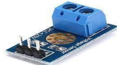
Figure 4: Voltage sensor module.
