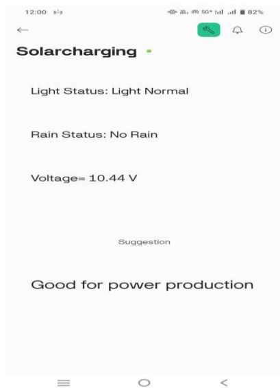
Figure 10: Dashboard state under normal light with no rain; recorded terminal voltage 10.44 V, classified as suitable for power production.
