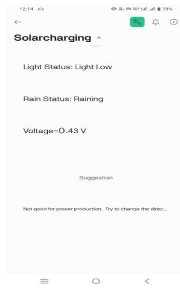
Figure 11: Dashboard state under low light with rain; recorded terminal voltage 0.43 V.
