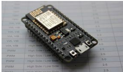
Figure 2: NodeMCU ESP8266 development board used as the system controller.
