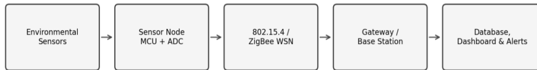
Figure 1. Proposed WSN-based environmental monitoring system architecture
