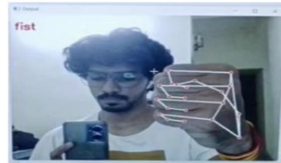
Fig.7. Recognized fist gestures of the hand and verified as the fist signal.
