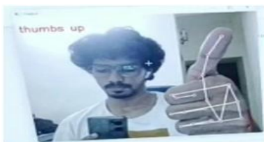
Fig.5. Recognized thumbs up gestures of the hand and verified as the thumbs up
