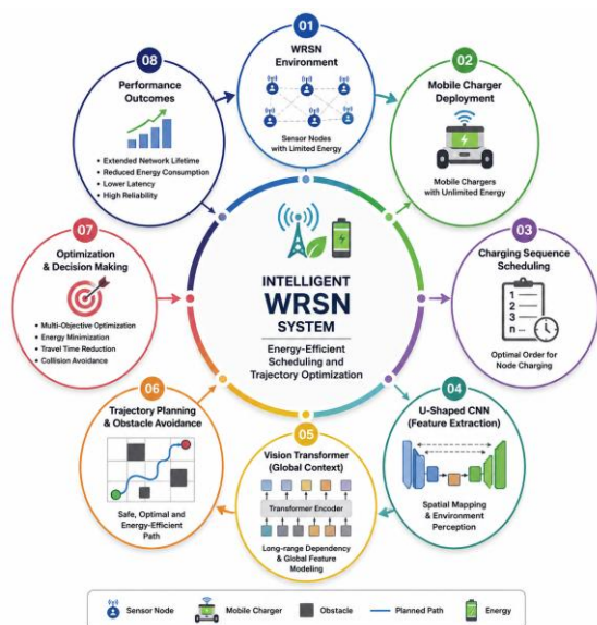
Figure 1. Intelligent WRSN Framework for Energy-Efficient Charging Scheduling and Trajectory Optimization
