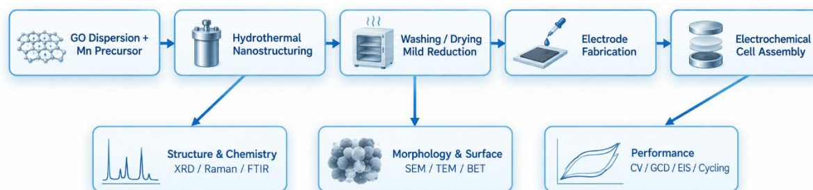
Figure 1. Proposed synthesis-to-electrochemical-performance workflow for nanostructured energy-storage electrodes.
