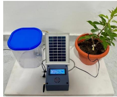
Fig (i): GSM DTMF Based Smart Irrigation System Working On Renewable Energy
