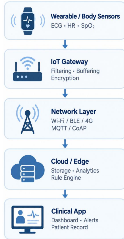
Figure 1. Proposed architecture for performance evaluation of an IoT-enabled smart healthcare monitoring system.
