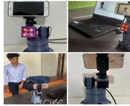
Figure2. Gimbal Control for Vision-based Target Tracking
