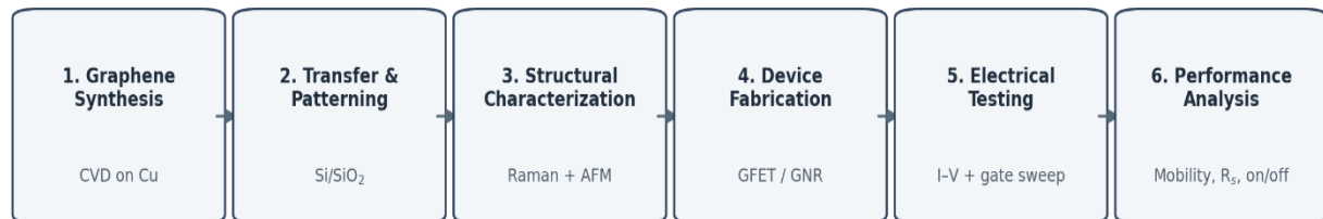
Figure 1. Proposed integrated workflow for graphene synthesis, characterization, device fabrication, electrical testing, and performance analysis. (Original schematic prepared for this methodology paper.)
