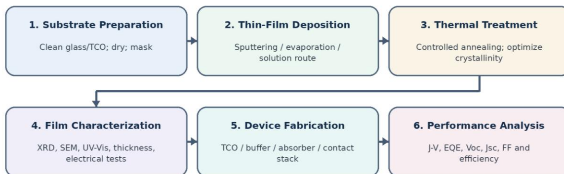
Figure 1. Step-by-step workflow for analysis of semiconductor thin films for photovoltaic applications.
