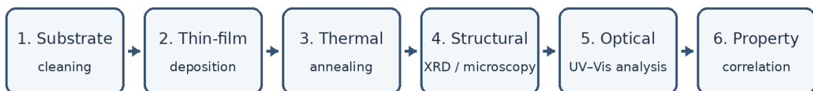
Figure 1. Proposed workflow for preparation, structural characterization and optical analysis of semiconductor thin films.
